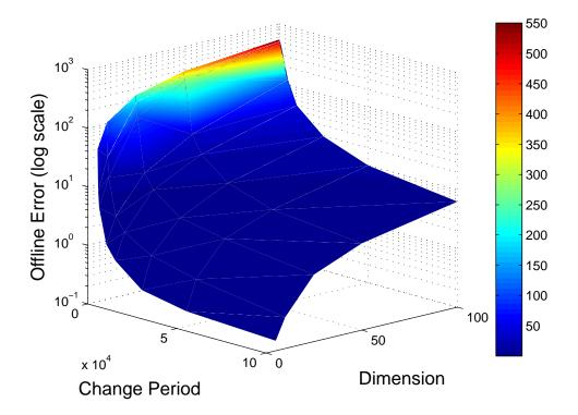
Figure 4.7: Offline error of DynDE on the MPB using the conical peak function with change severity 1.0 for various settings of number of dimensions and change period.
